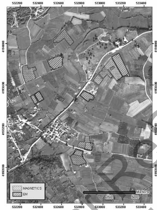
Fig. 1. WorldView Satellite image of Elis outlining areas covered with magnetic and electromagnetic geophysical mapping methods
